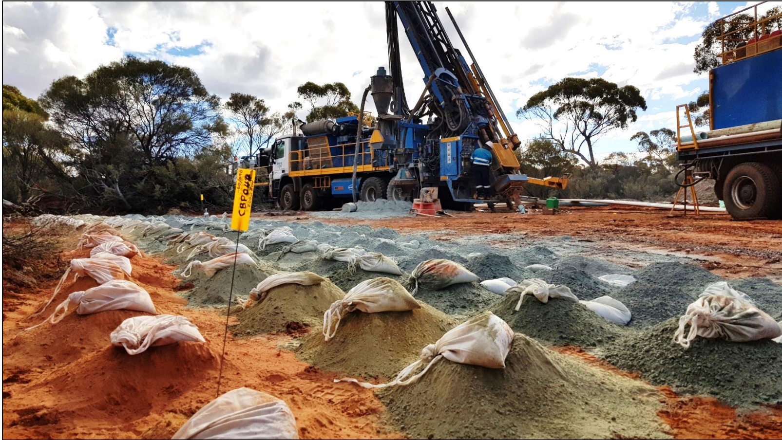
2019 RC drilling operations at Carr Boyd Nickel Project
