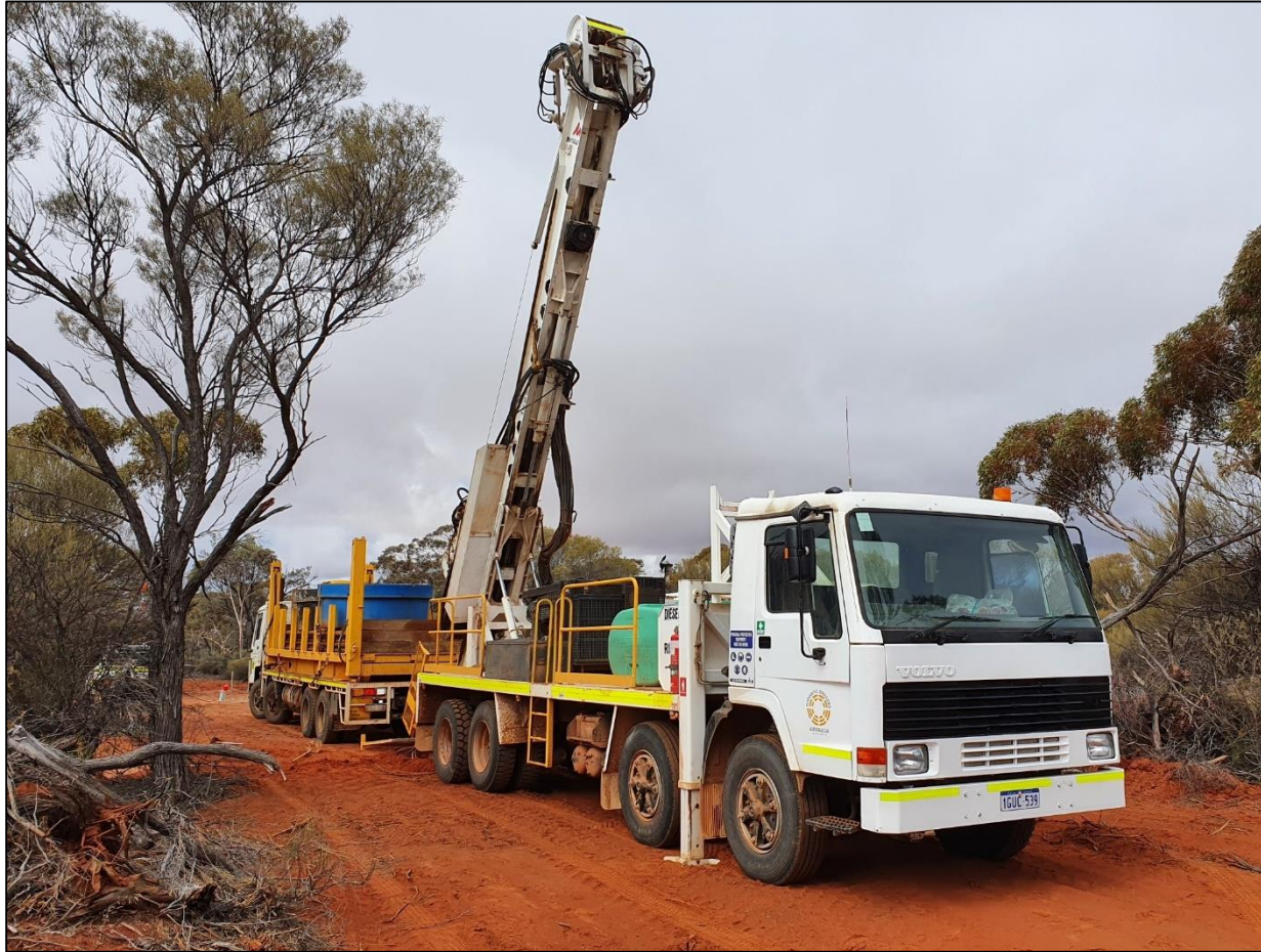
Aug 2020 Diamond drilling operations at Carr Boyd Nickel Project
