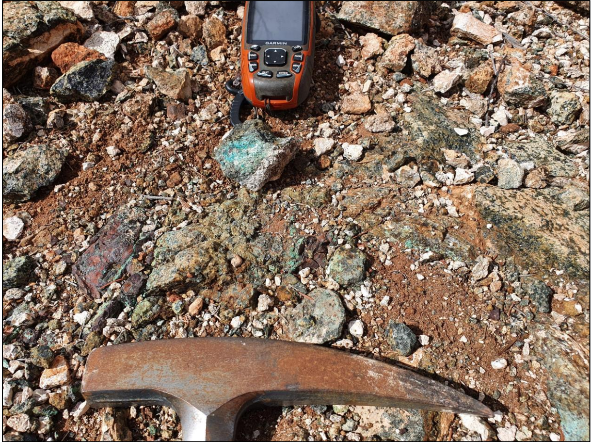
Figure 2. Copper oxide minerals (green-blue) and gossanous sulphides (dark brown) mineralisation in shallow scrapings/pits at POH prospect (368961E/6674000N)
