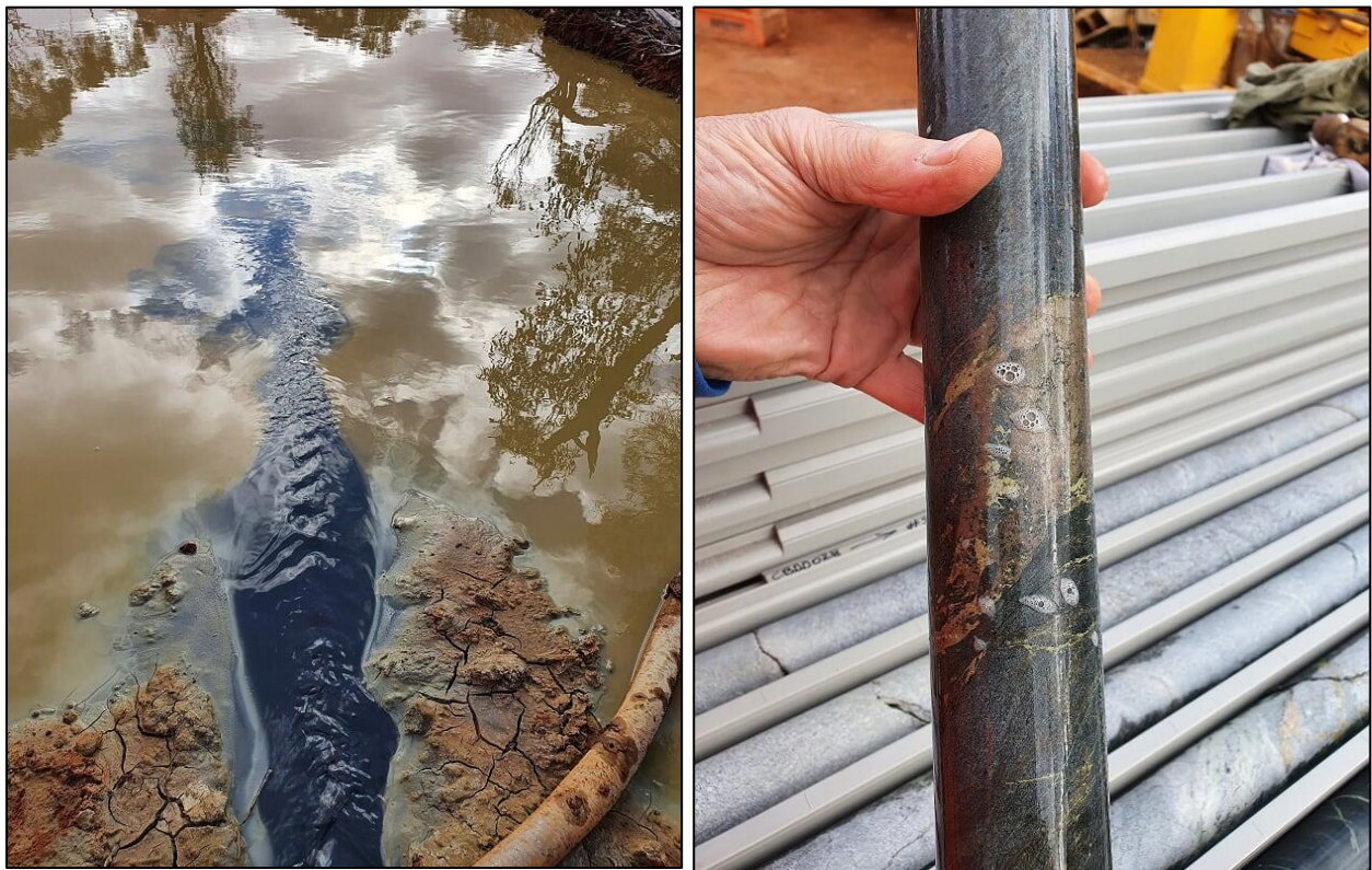
Figure 1. Drilling water turns black as Ni-Cu sulphides (pyrrhotite-pentlandite-chalcopyrite) are intersected in diamond drill hole CBDD0028 at the T5 Ni-Cu discovery zone (165m-165.5m shown).
