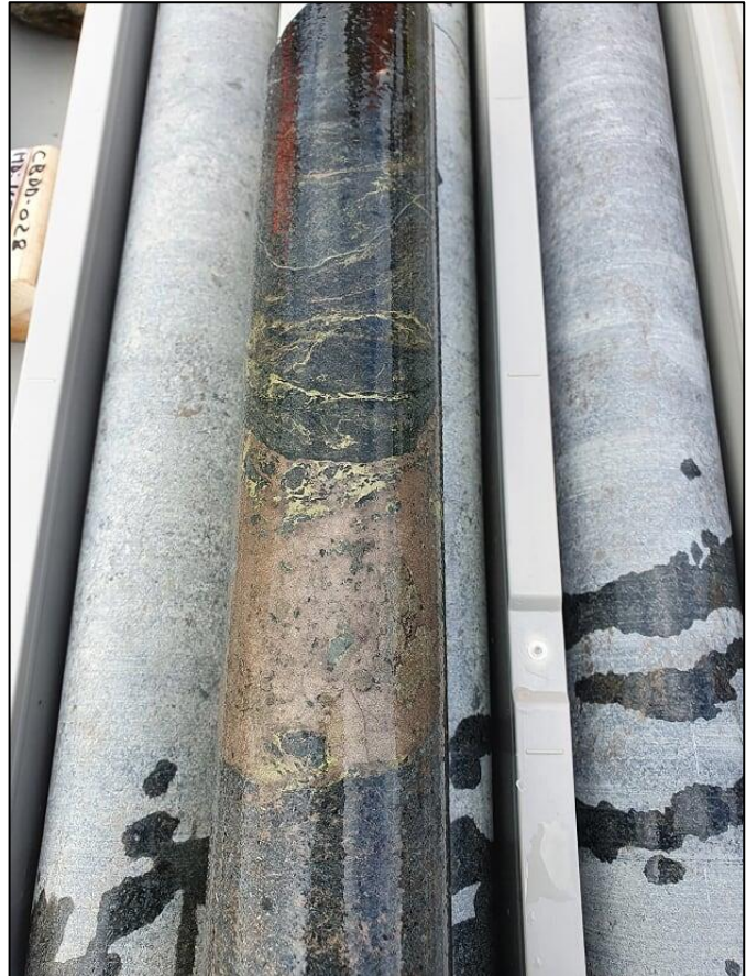
Figure 2. Semimassive and matrix style Ni sulphides (bronze colour) with stringer Cu sulphides (golden colour) in drill core (165m-165.5m shown).
