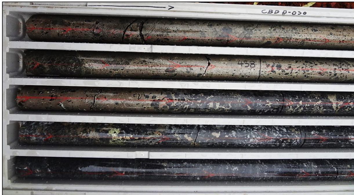
Figure 5: Unique magmatic sulphide textures in CBDD0030 showing breccia clasts within the massive sulphide, interstitial sulphide/crystal intergrowth at the margin, and chalcopyrite segregation within the crystallised host pyroxenite.
