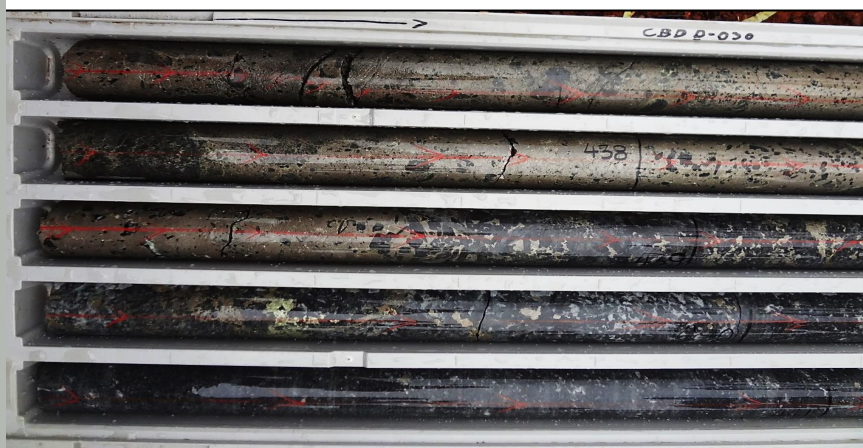
Figure 1: High grade nickel sulphides showing cumulate magmatic sulphide textures within the main massive-matrix sulphide zone. The mineralisation comprises breccia clasts within the pyrrhotite-pentlandite-chalcopyrite sulphides, interstitial sulphide/crystal intergrowth at the margins and chalcopyrite segregation within the crystallised host pyroxenite. Coarse blebs of matrix sulphide are observed between the crystallising host rock. (CBDD0030 - 436.7m-441.1m shown). This zone is interpreted as one of several feeder zones within the CBIC.
