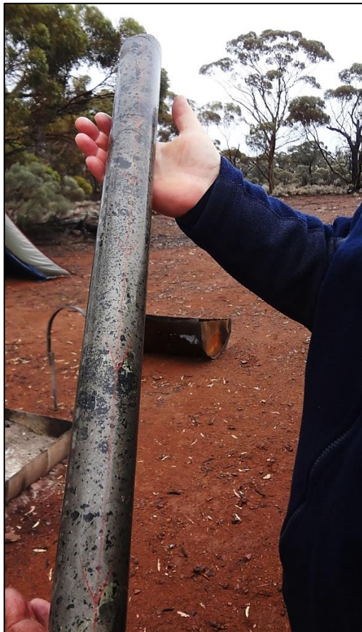
Figure 3: Ni-Cu bearing massive sulphide zone in diamond drill hole CBDD0030 (436.7m-437.6m).
