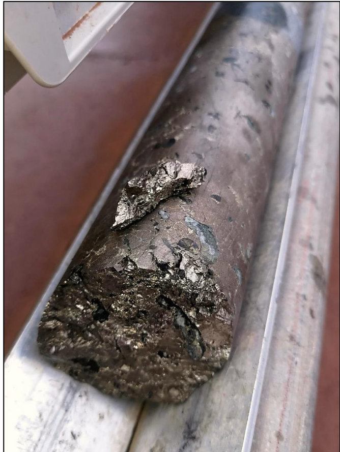
Figure 4: Close-up of sulphides from CBDD0030
