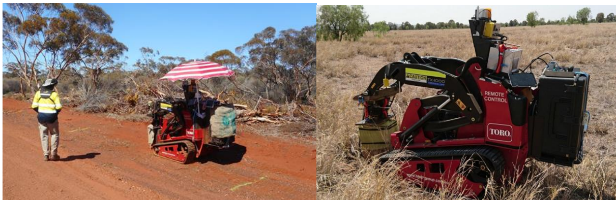
Figure 7: R&D Seismic Survey conducted by Ultramag enabled very low environmental impact seismic surveying at Carr Boyd, allowing the company to image the prospective basal contact at depth ahead of drill planning. The e-Vibe system enable access into areas where traditional seismic systems would be too large and destructive to operate effectively.
