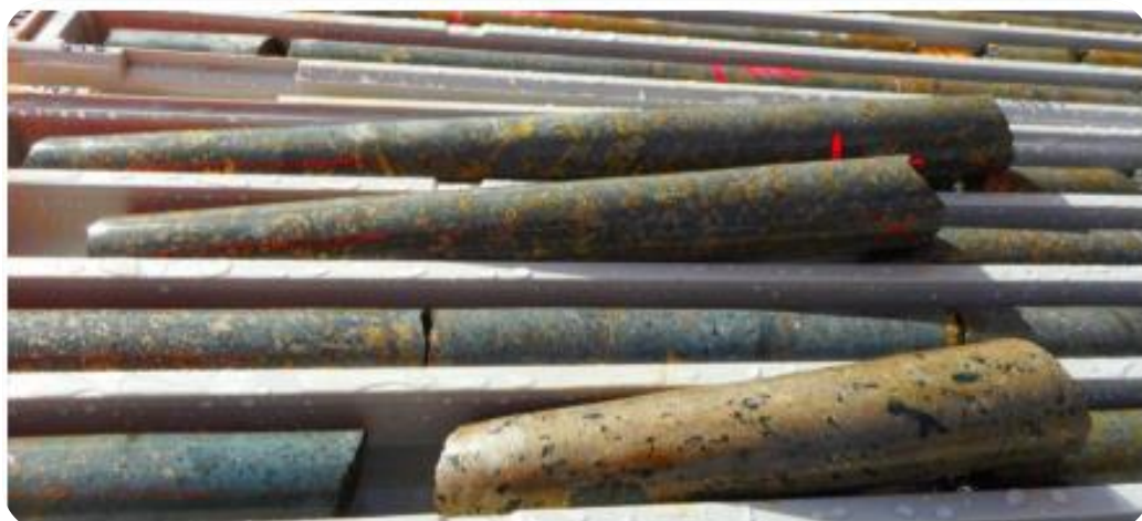
Massive and globular nickel-copper-iron sulphide breccias in CBDD054B at 368m
