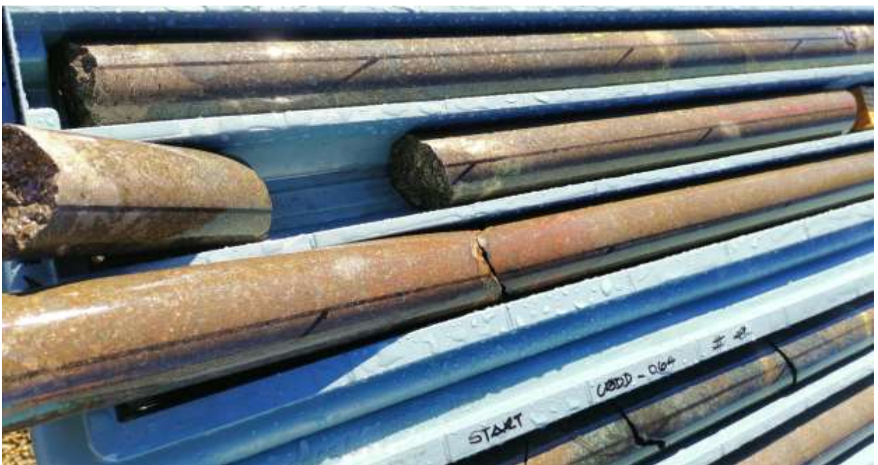
➔ Figure 1: Massive and semi-massive nickel-copper sulphides in CBDD064 at ~198m downhole.
