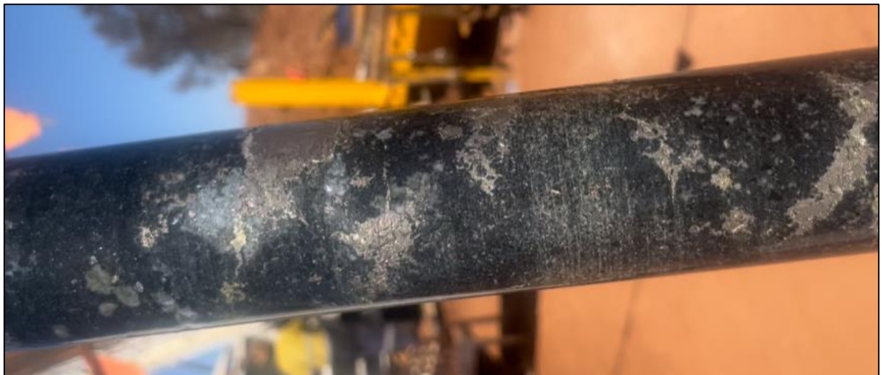
Figure 1: Diamond core with globular nickel-copper sulphides at approximately 802m downhole in CBDD067.
